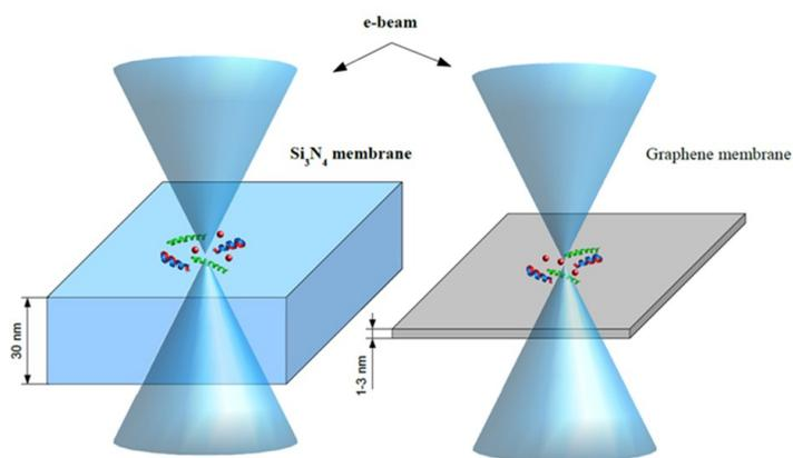
3. Thickness comparison of a silicon nitride TEM grid (left) to a graphene TEM grid (right).
