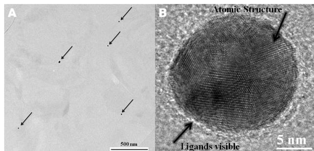
2. (A) Low resolution TEM image of gold nanoparticles with arrows pointing towards them on a graphene film. (B) A high resolution image of gold nanoparticles on a graphene film. The gold atomic structure and ligands are visible. The graphene films used were from the Graphene Supermarket, courtesy of Professor Bolotin, Vanderbilt University.
